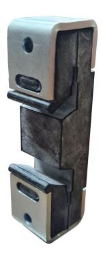
EasyGrip Sound Isolation Clips resiliently secures common drywall furring channel Offering significantly higher STC values than drywall attached to resilient channel, EasyGrip ensures that installers will not inadvertently screw through the "resilient" leg of the channel into the joist or stud.
