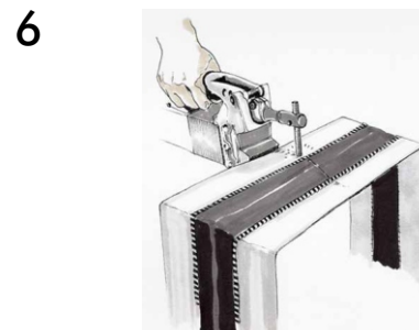
Spotweld the steel and form to the desired shape
